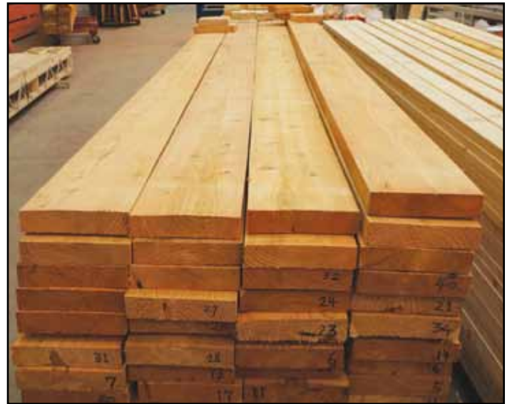
Figure 13: 225mm deep C24 larch from Wentwood forest at Fforest Timber Engineering
