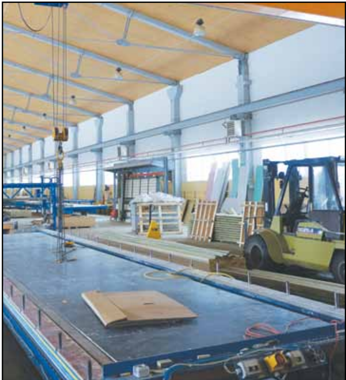
Figure 21: Closed panel production line in Latvia with overhead crane and butterfly tables
