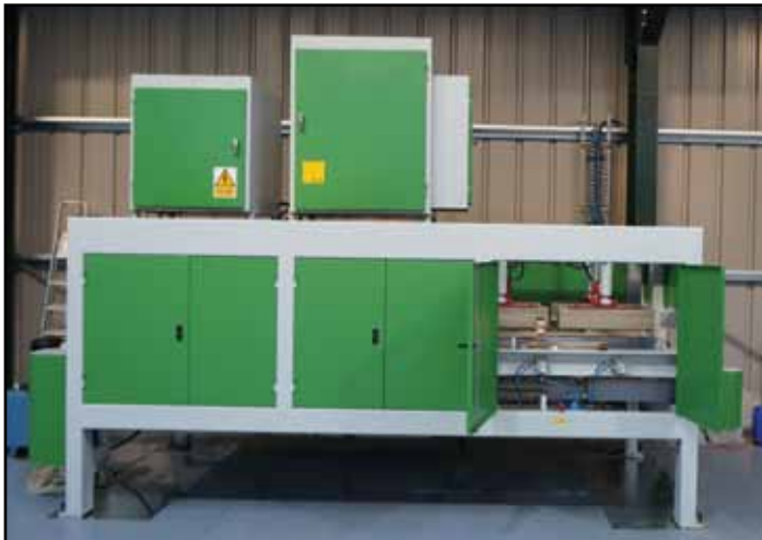
Figure 34: The new radio frequency high volume glulam press at Clifford Jones Timber, Ruthin
