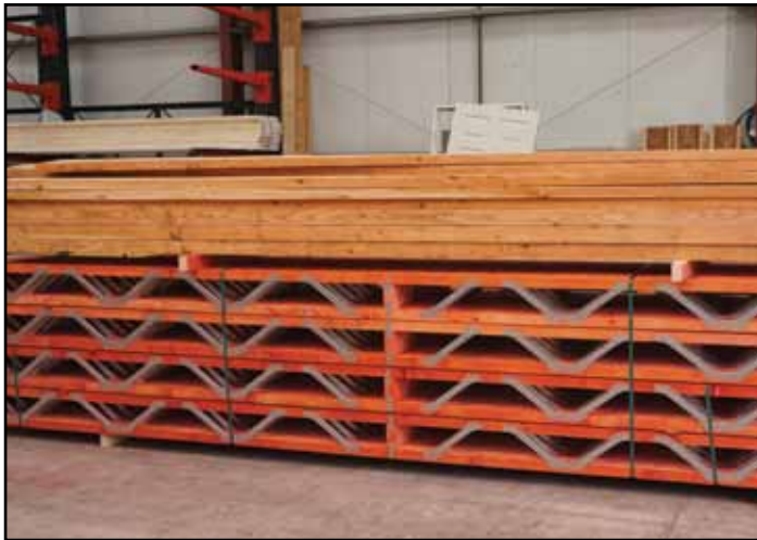
Figure 35: Posi-joists at Fforest Timber Engineering - these could utilise Welsh softwoods now
