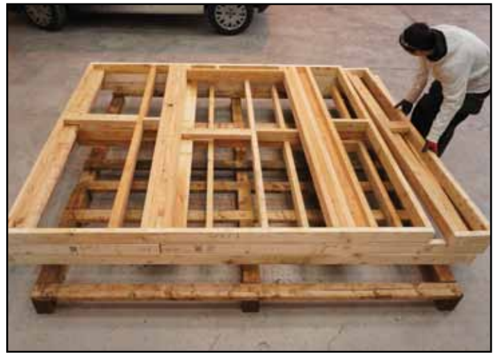
Figure 12: Welsh larch assembled as partly complete open panels at Fforest Timber Engineering
