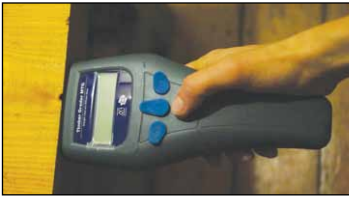
Figure 2: The Brookhuis MTG hand held acoustic grading tool
