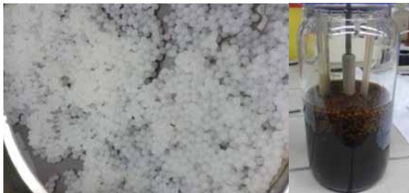
Fig. 9. (A) Immobilized A. succinogenes cells in alginate beads and (B) the bioreactor system used
