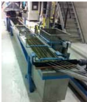
Fig.11. Picture of the compounding process at industrial scale for a blend of PHB/PBS with FR additives.
