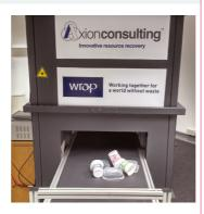
that can be scanned by a laser to reflect a specific pattern. The image is photographed and then analysed by a recognition system. It is the first time such a concept has been used in this type of sorting application – it worked well and could "revolutionise" any food contact plastic recycling, according to Axion.
