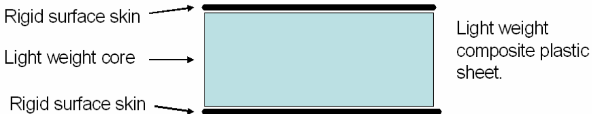
Figure 16 Scheme of a sandwich foamed material
